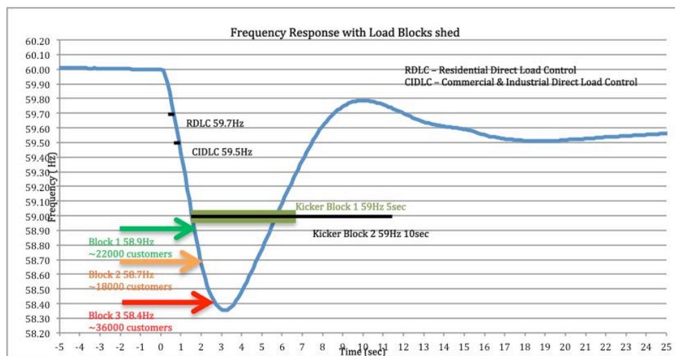
Figure 4-21. Frequency Response with Load Blocks Shed
