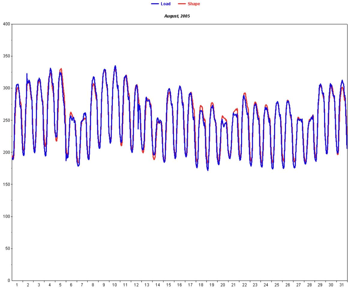
Figure 49: Actual (Blue) and Predicted (Red) System Hourly Load (MW)
